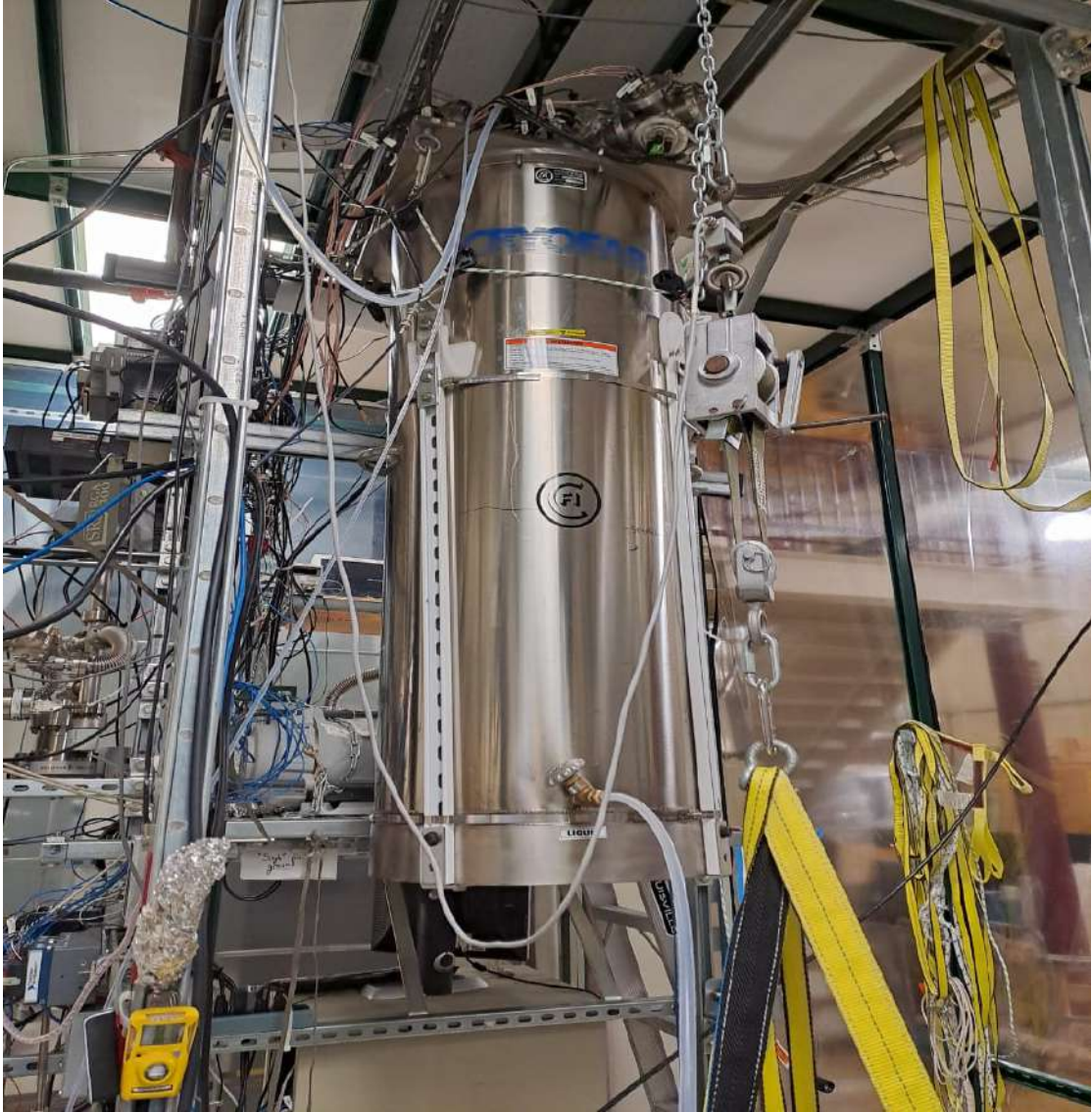
FIGURE 3.3: The TPC dewar filled with HFE-7000.
