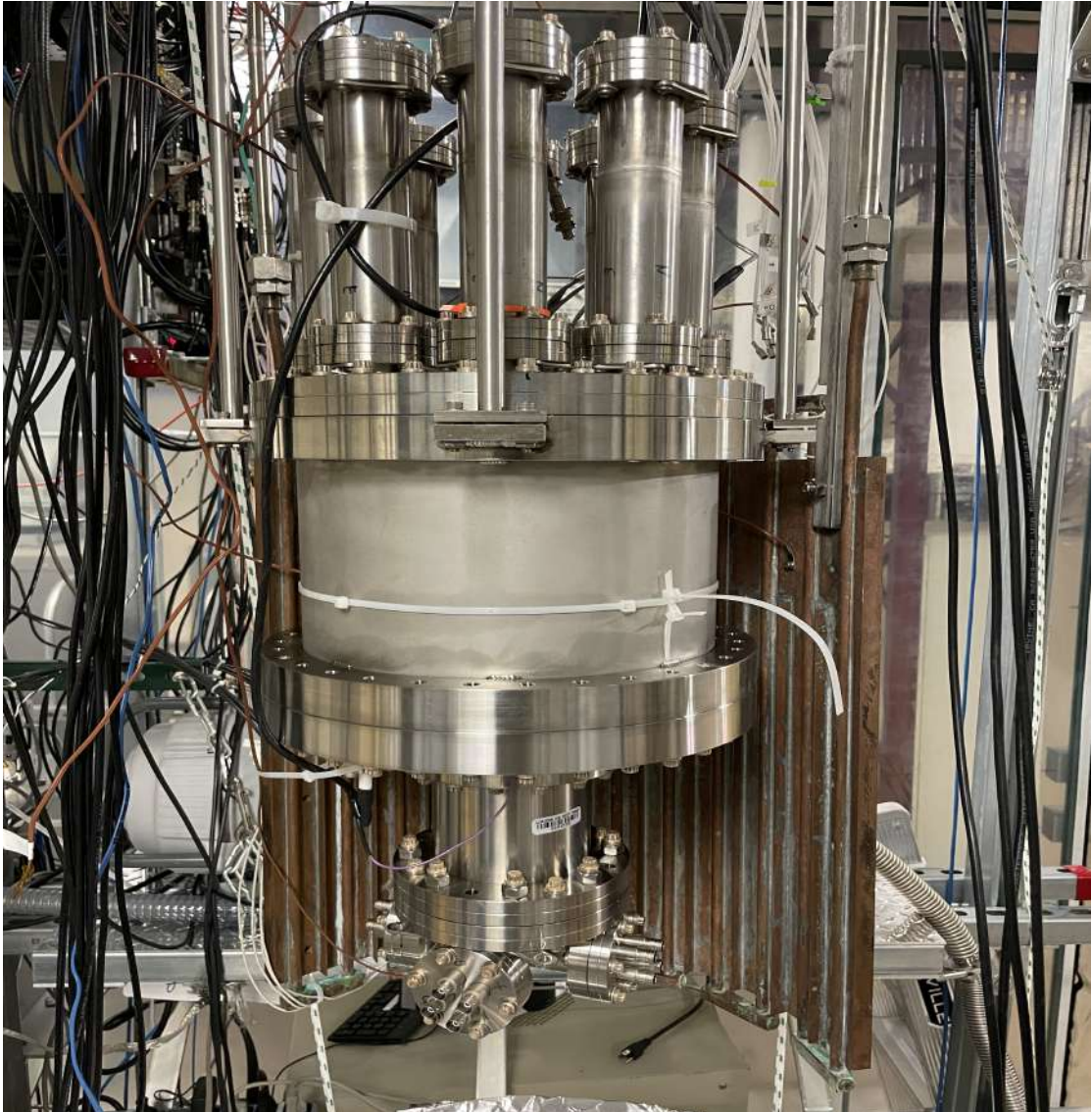
FIGURE 3.1: The cylindrical stainless steel chamber that contains the TPC and the semi-cylindrical copper plate that surrounds the TPC.
